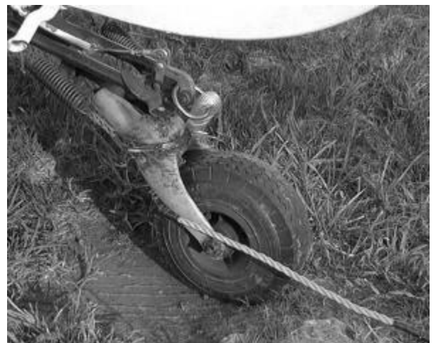
Bad Tow plane Rope Condition
