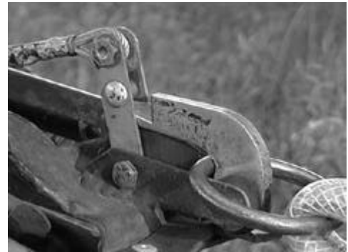
Bad Tow plane Hook Condition Notice arming lever slanted to left
